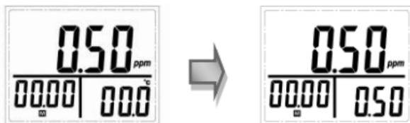
Press button **SEL** or **MAX/MIN** to adjust the value of main window to 0.5ppm.
